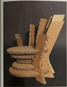
In this more resistant model I included less backs as the cardboard kept bending and the cardboard between the different backs wasn't strong enough. To improve the design I need to make the inner circle bigger to make sure It fits all the slots. I kept the curves and considered making the backs more upright but I decided that that would take away from the design and make It less fluid.
