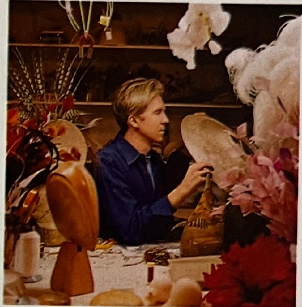
Treacy makes prototype forms in a light flexible material called Sparterie. Sparterie is often known by referred to as willow by Milliners, the open weave grass cloth bonded to a fine cotton gauze by starching, so the top becomes softer both in appearance and texture. Treacy then sends these initial forms to a Parisian blockmaker at La Forme who carves them out of beechwood. Beechwood is used as its softness allows pins to be stuck in it and mould materials onto the wood.
