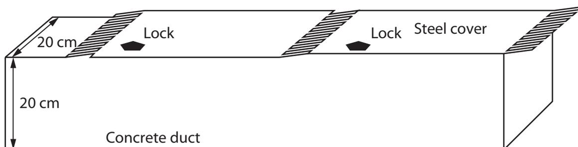
All of the service ducts have water pipes and mains (240v) electricity cables running through them. Other services such as a gas supply or telephone cable are installed when needed. This makes the system very flexible.
