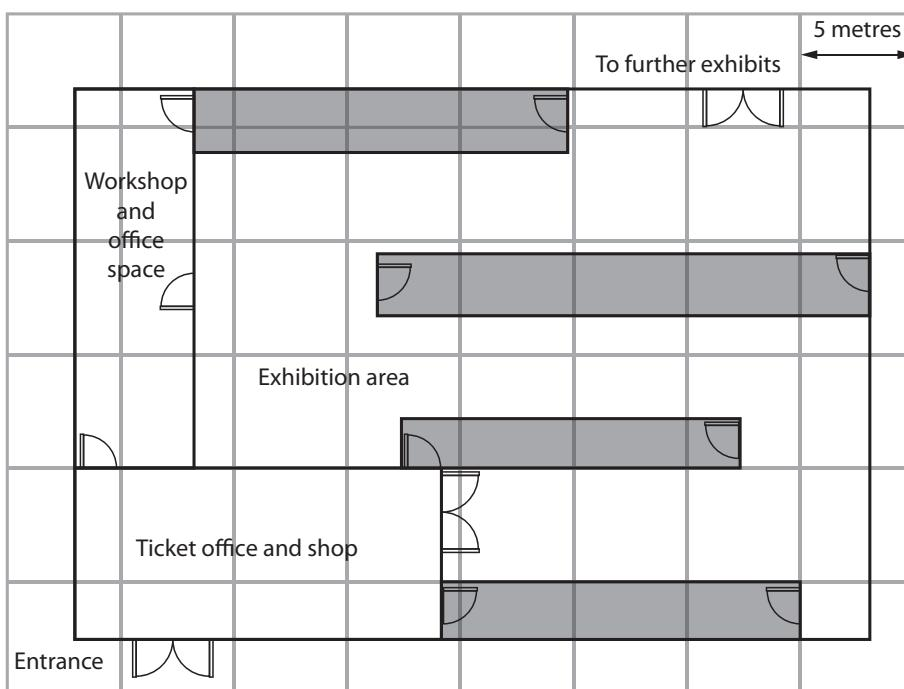
The areas shaded in grey are for staff only and are used for setting up and servicing the exhibits. These areas are open at the top and have internal ladders to allow access to the service grid.
