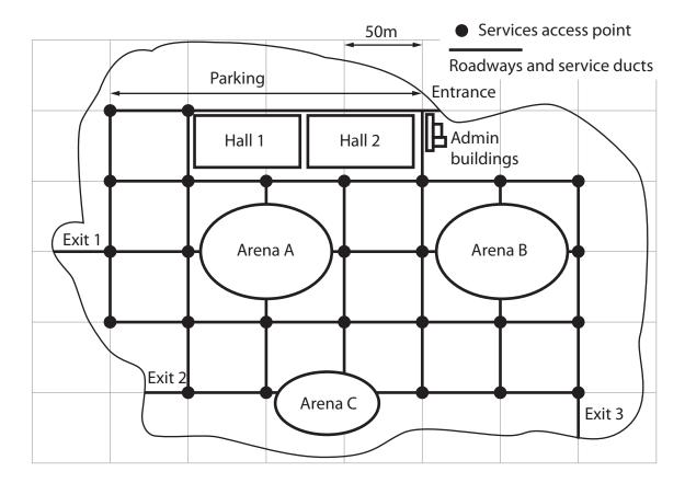
There are service ducts running beside the roadways. These consist of 20 cm square concrete channels with lockable steel covers. The covers are in one metre lengths with flexible rubber at each end. This allows easy installation of cables and pipes. You may assume that Hall 1, Hall 2, and the admin buildings have connections to the service ducts wherever they are required.
