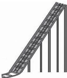
The first part of the ride will be a powered climb. The cart is linked to a chain which is driven by a powerful motor. This drives the cart up to the top of the Powered Climb where it is released by the chain and the cart starts its gravity driven ride. As you are only allowed **ONE** powered climb and this must be at the beginning of the ride it should take you to the **HIGHEST** point of the ride.
