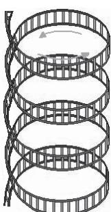
The Spiral is a series of sharp  $360^\circ$  turns, one after the other, going downwards. The effect of the feature is to make you feel as if you are being thrown sideways out of the cart. This cannot happen of course but considerable lateral g-force is felt.
