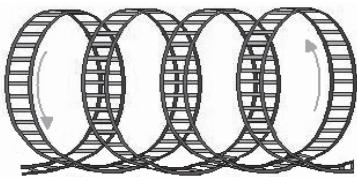
The Corkscrew is a cross between the Loop and the Spiral. It looks like a spiral on its side but turns the cart upside down several times in quick succession.
