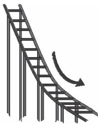
The Drop is the opposite of a climb. The track simply turns downward. This feature is mainly used to build up speed. The ride will be dangerous if the cart doesn't gather enough speed to negotiate some features.
