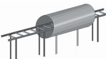
The Tunnel is a horizontal ride through a dark covered area. The height of the covered area is designed to be high enough to be safe but low enough to make the passengers think they have to duck.
