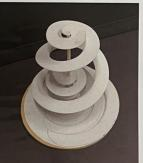
Inspired by Ron Arad's Geoff sphere I started experimenting with laser cutting spiral patterns. These models are simple linear spiral patterns. The second model has smaller spirals inside the larger one so it is more condensed where the light would be. Also this creates an interesting pattern. However these spirals are very open so I could have multiple spirals of the same size to hide more of the centre.
