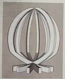
This chair still follows the x seat style. However instead of doing this using each piece of the frame running parallel as the one above does the lines are perpendicular and meet in the middle crossing over. This takes away the old-fashioned design and gives it a modern twist. Also, I have used a similar curved base however instead of it stopping at the arm rest it curls right the way round creating the cocoon shape.
